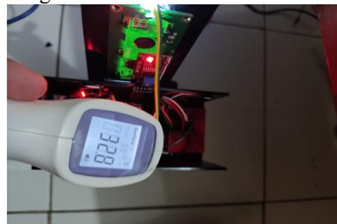
Gambar 18. Pengukuran Suhu IC Regulator Arduino
